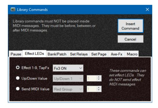
In addition to setting effect LEDs off and on, you can control LEDs for the Stepper and Send MIDI groups. None of these options sends MIDI messages associated with these effects, they only affect LEDs.
