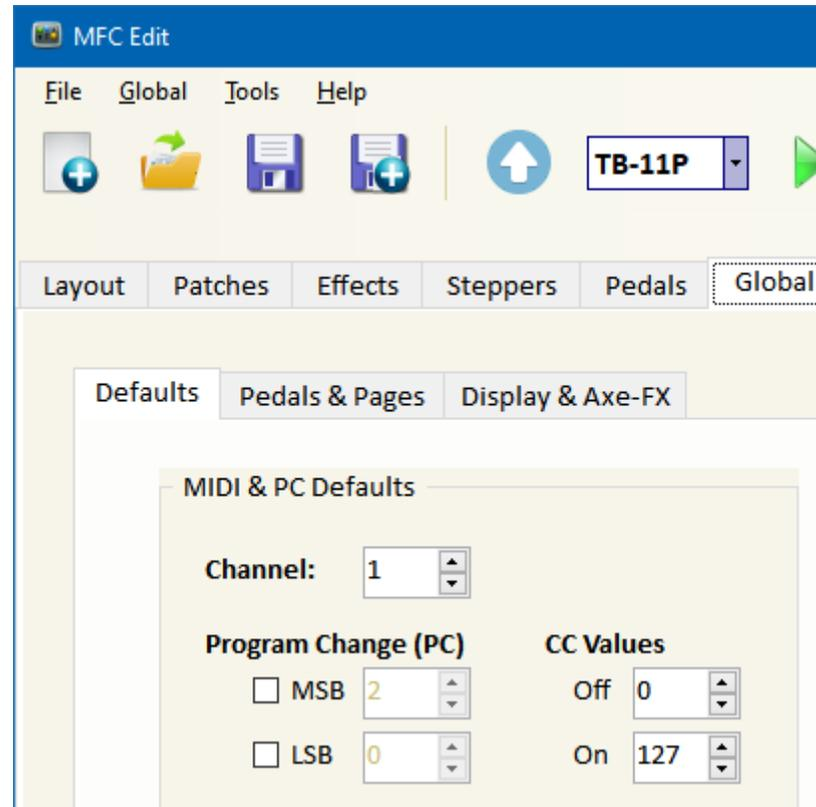
3. Select the Global Pedals tab and check your connected pedal types are correct. It's important to set this before assigning pedals later on the Layout tab.
