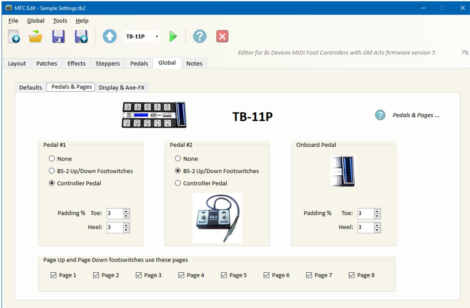
The screenshot shows the MFC Edit software interface for configuring a TB-11P MIDI Foot Controller. The window title is "MFC Edit - Sample Settings.tb2". The menu bar includes File, Global, Tools, and Help. The toolbar contains icons for file operations, a dropdown menu set to "TB-11P", and help/exit buttons. The status bar indicates "Editor for BJ Devices MIDI Foot Controllers with GM Arts firmware version 5" and "7%".
