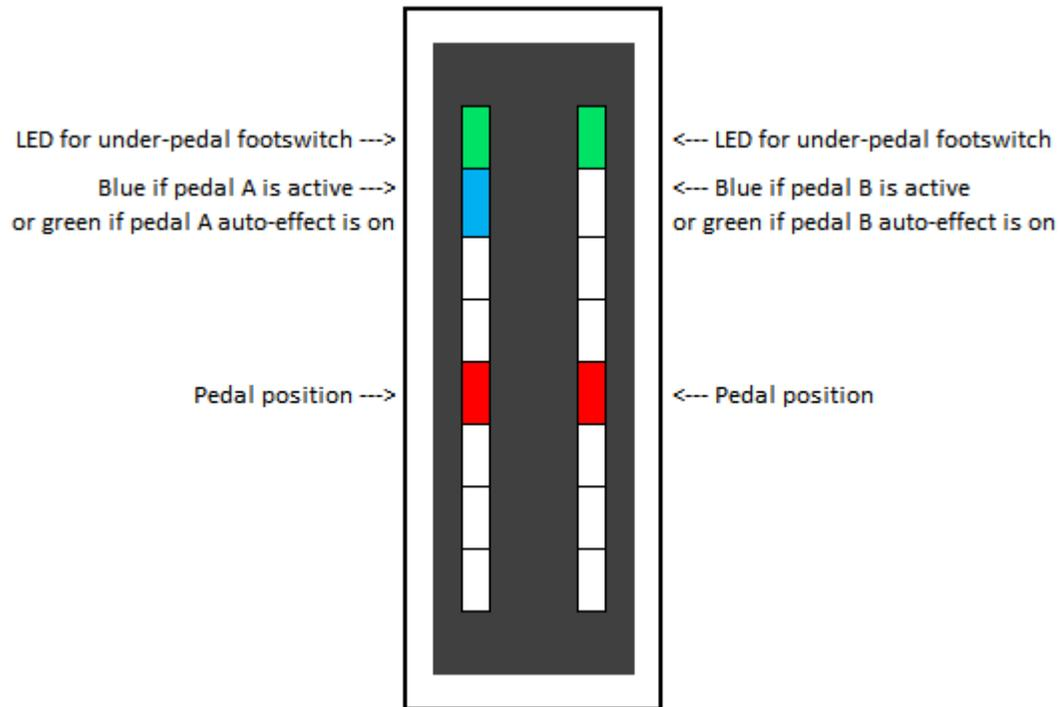
The pedal position LED is blue by default, but you can assign a page LED colour of your choice to the pedal.
