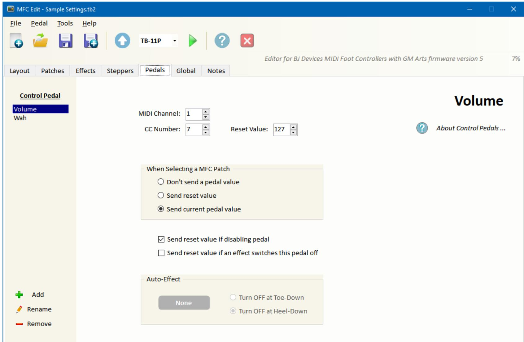
MFC pedals can be disabled on the MFC itself which is useful if a pedal cable fails for example. There is an option to send the reset value if disabling the pedal. Also, an effect can turn a pedal function off when switching between A and B pedals. You can choose to send the reset value when that happens.
