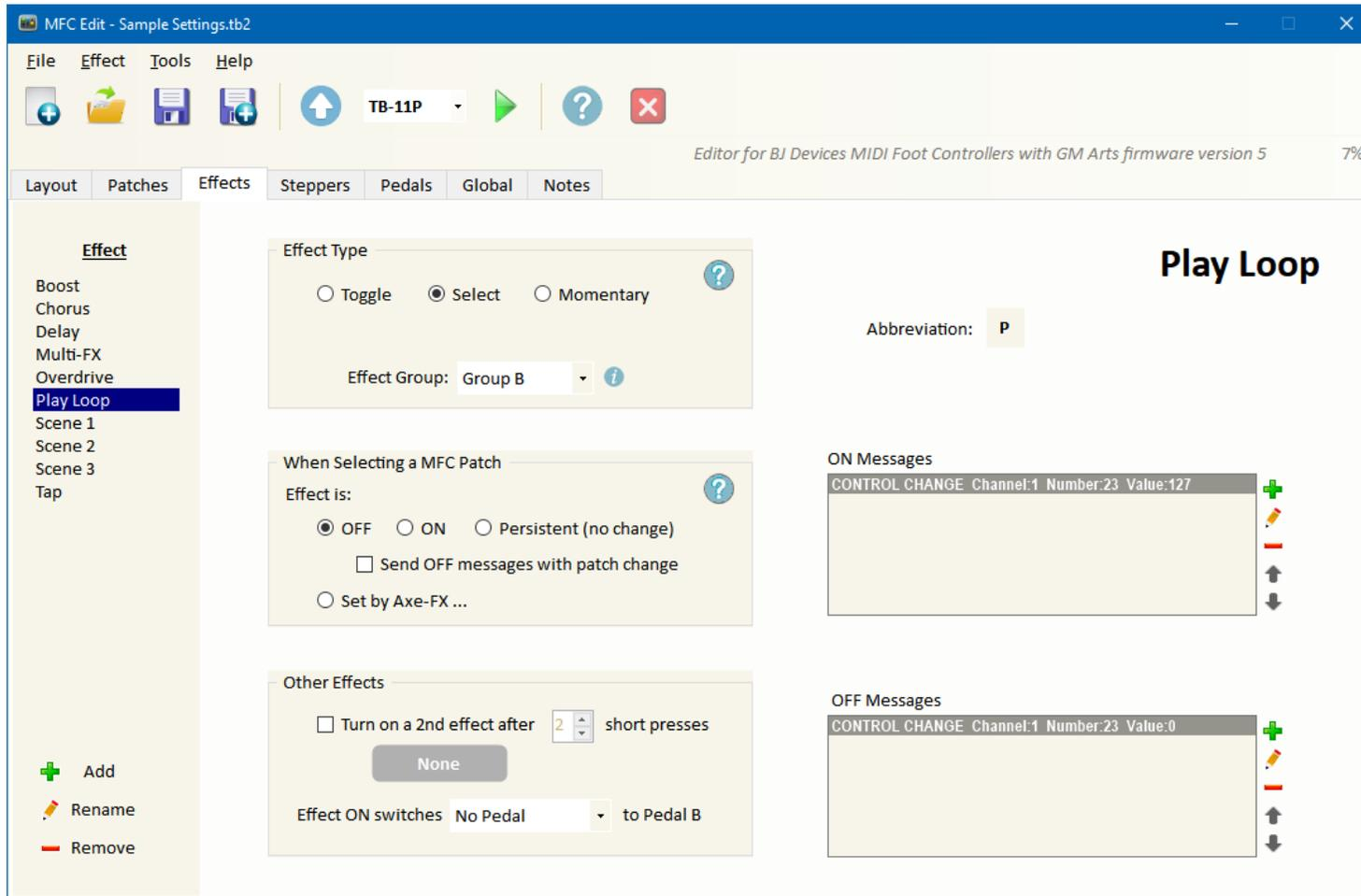
Because you can use the ON and OFF messages to send any CC values you want, you can also set effects to work in reverse. For example you might use an EQ effect to cut mids and volume level for a rhythm sound, but you want it to show as ON for soloing when the effect is off. Check "Display OFF as ON" to reverse the footswitch LED and abbreviation displays. This applies only to toggle effects that are not in a group.
